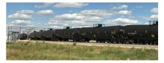
of the Bakken Oil Express. The actual entrance is located at 3761 115th Ave. SW, but this position allows you to see the connecting infrastructure. It opened in October of 2011 and is connected to the Four Bears/ Belle Fourche regional pipeline system. BOE is a 4-loop track facility capable of simultaneously loading two trains and has storage for 640,000 barrels on site.
